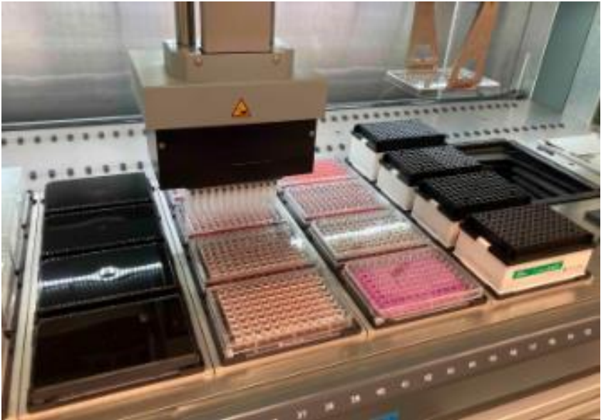
State-of-the-art, integrated system for screening gene circuit libraries in one continuous process within primary human NK cells
